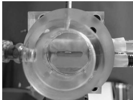
Figure 3: The artificial mouth used in double-reed measurements
