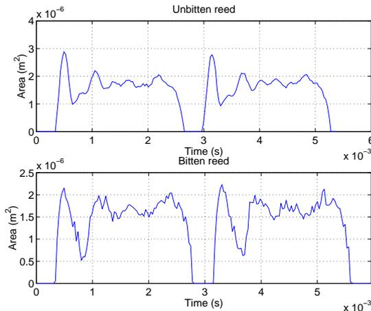
FIG. 10: Opening area measurements on a real unbitten and bitten reed.
