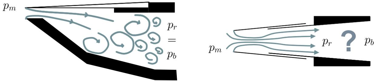
FIG. 1: Flow inside clarinet and oboe embouchures
